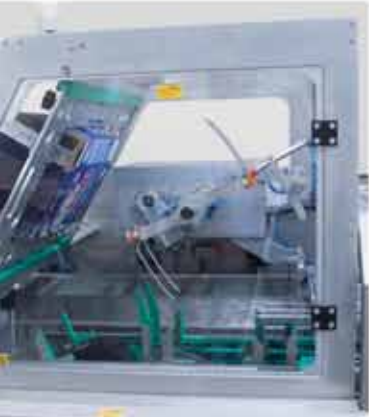
Servomotor Tahrikli 3 İstasyon Kutu Açma Servomotor Driven 3 Station Box Erecting
