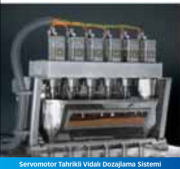
Servomotor Tahrikli Vidalı Dozajlama Sistemi Individually Servomotor Driven Auger Dosing System
